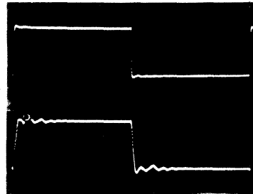
TOP TRACE: INPUT - 50mV/DIV - 1 μsec/DIV BOTTOM TRACE: OUTPUT - SAME SCALE
